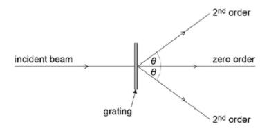
The grating is then replaced by a plane transmission grating which has 2N slits per metre.
