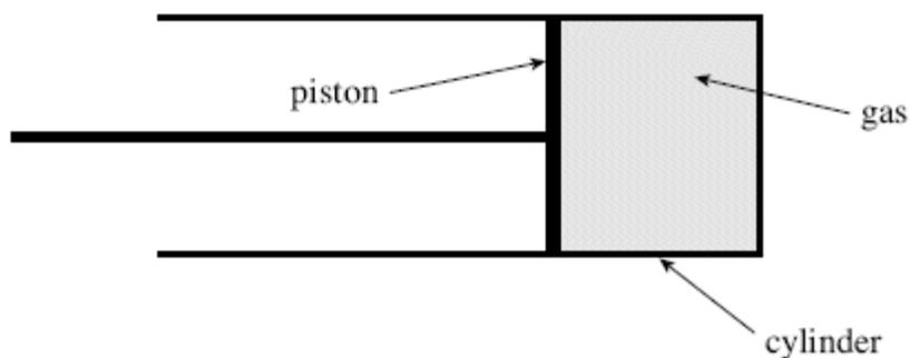
**Figure 1** shows a cylinder, fitted with a gas-tight piston, containing an ideal gas at a constant temperature of 290 K. When the pressure,  $p$ , in the cylinder is  $20 \times 10^4$  Pa the volume,  $V$ , is  $0.5 \times 10^{-3} \text{ m}^3$ .
