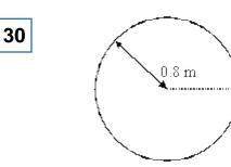
A model car moves in a circular path of radius 0.8 m at an angular speed of  $\frac{\pi}{2}$  rad s<sup>-1</sup>.
