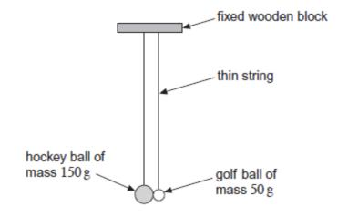
A golf ball of mass 50 g is initially hanging vertically and just touching a hockey ball of mass 150 g. The golf ball is pulled up to the side and released. It has a speed of 1.3 m s<sup>-1</sup> when it collides head-on with the hockey ball. After the collision the balls move in opposite directions with equal speeds of 0.65 m s<sup>-1</sup>.
