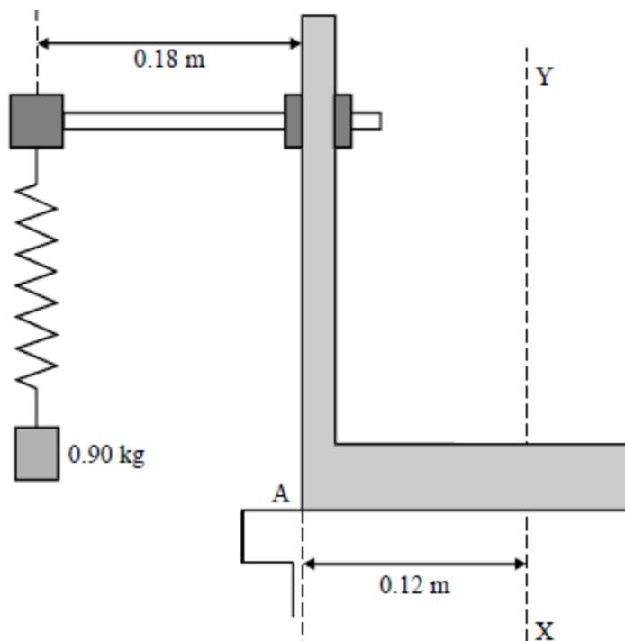
The mass of a retort stand and clamp is 1.6 kg and their combined centre of mass lies along the line XY. A spring which has a negligible mass is attached to the clamp and supports a mass of 0.90 kg, as shown in the diagram. The spring requires a force of 6.0 N to stretch it 100 mm.
