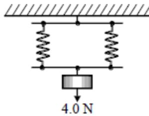
The spring constant of each spring is  $20 \text{ N m}^{-1}$ . The elastic energy, in J, stored in the system is
