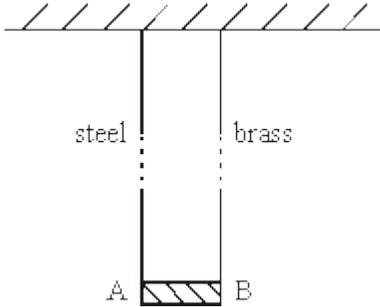
When a mass of 16 kg is suspended from the centre of AB, the bar remains horizontal.
