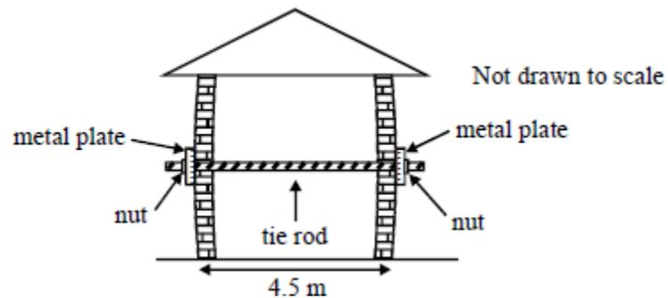
In one case a steel tie rod of diameter 19 mm is used as shown above. When the nuts are tightened, the rod extends by 1.5 mm. The Young modulus of steel is  $2.1 \times 10^{11}$  Pa.
