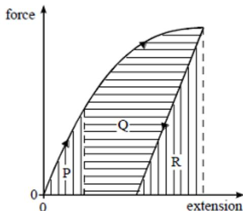
The increase in thermal energy in the sample is represented by area
