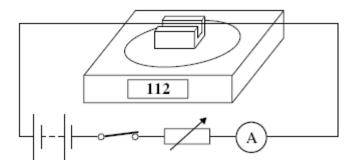
The balance, which was zeroed before the switch was closed, reads 112 g after the switch is closed. If the current is reversed and doubled, what will be the new reading on the balance?
