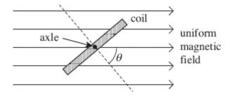
A coil of 50 turns has a cross-sectional area of  $4.2 \times 10^{-3} \text{ m}^2$ . It is placed at an angle to a uniform magnetic field of flux density  $2.8 \times 10^{-2}$  T, as shown in the diagram, so that angle  $\theta = 50^{\circ}$ .
