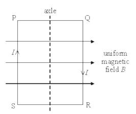
A coil, mounted on an axle, has its plane parallel to the flux lines of a uniform magnetic field *B*, as shown. When a current *I* is switched on, and before the coil is allowed to move,
