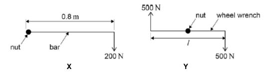
What is the minimum length l of the wrench which would be needed for him to loosen the nut?
